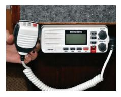
Your houseboat has come equipped with a VHF Marine Band Radio. It is located at the helm, to the right of the steering wheel.
