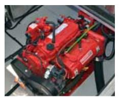
CAUTION: The blower must be used at least 5 minutes before starting the generator located below deck, to clear any fumes that may have collected.
